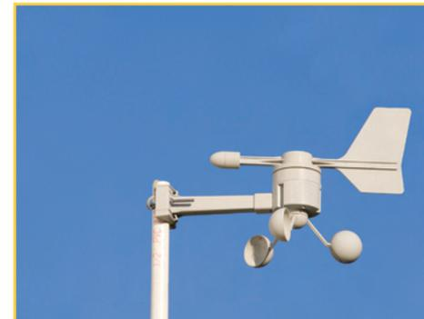
An anemometer should be used to measure wind speed over a year to gain an accurate picture of a site's wind resource.
