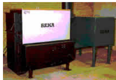
Moving grate 20 kW wood chip boiler with chip hopper
